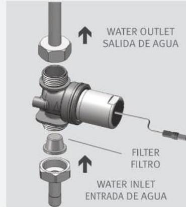
**(EN)** Note: Make sure the filter is located between the solenoid housing and the water inlet.
